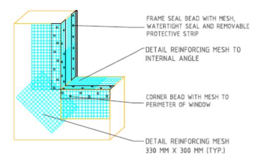
Figure 4b: Detailing of mesh around openings with corner beads
