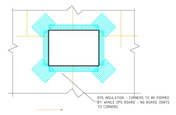
Figure 4a: Detailing of mesh around openings
