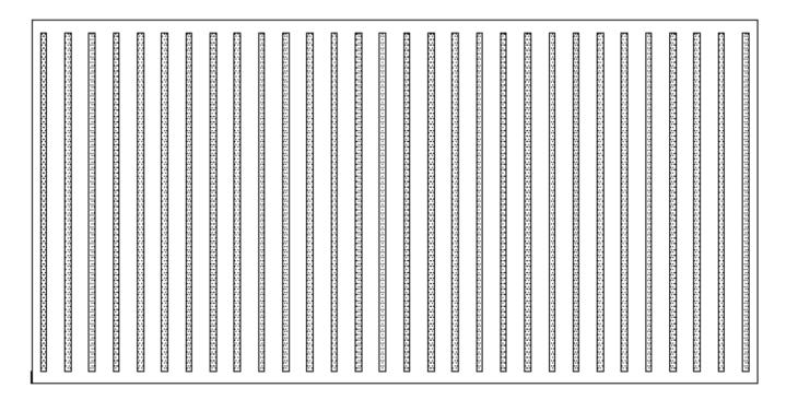
10MM WIDE NOTCHES 13MM DEEP SPACED @ 45MM CENTRES (VERTICAL)
