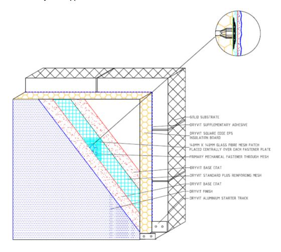
Figure 3a. Drysulation primary mechanical fix with supplementary adhesive with fixings through the mesh
